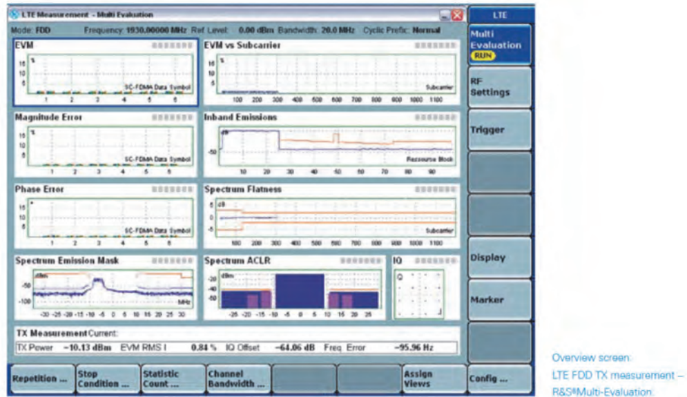
Figure 3.5: An example screenshot of an LTE FDD Transmit measurement on a Protocol Analyzer
